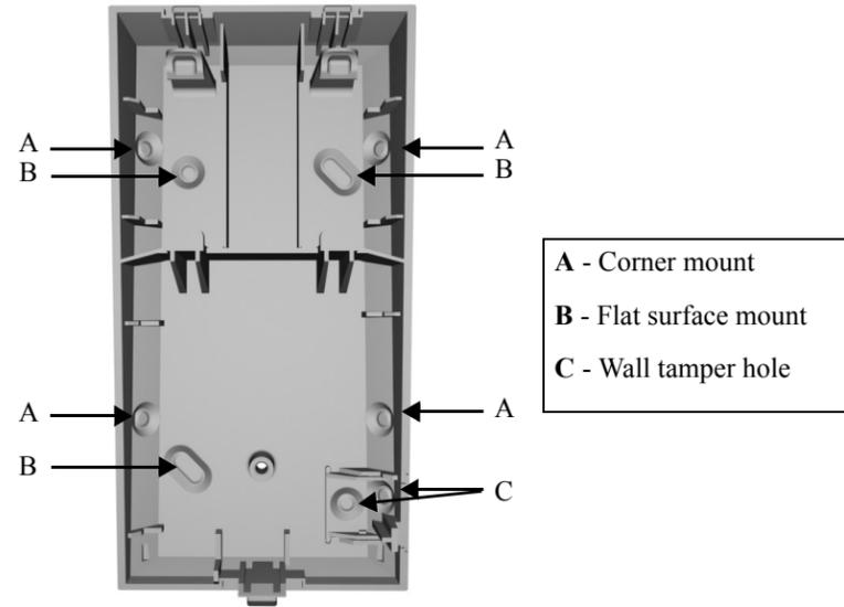
**Dual Tamper Mechanism - Wall and Cover**
